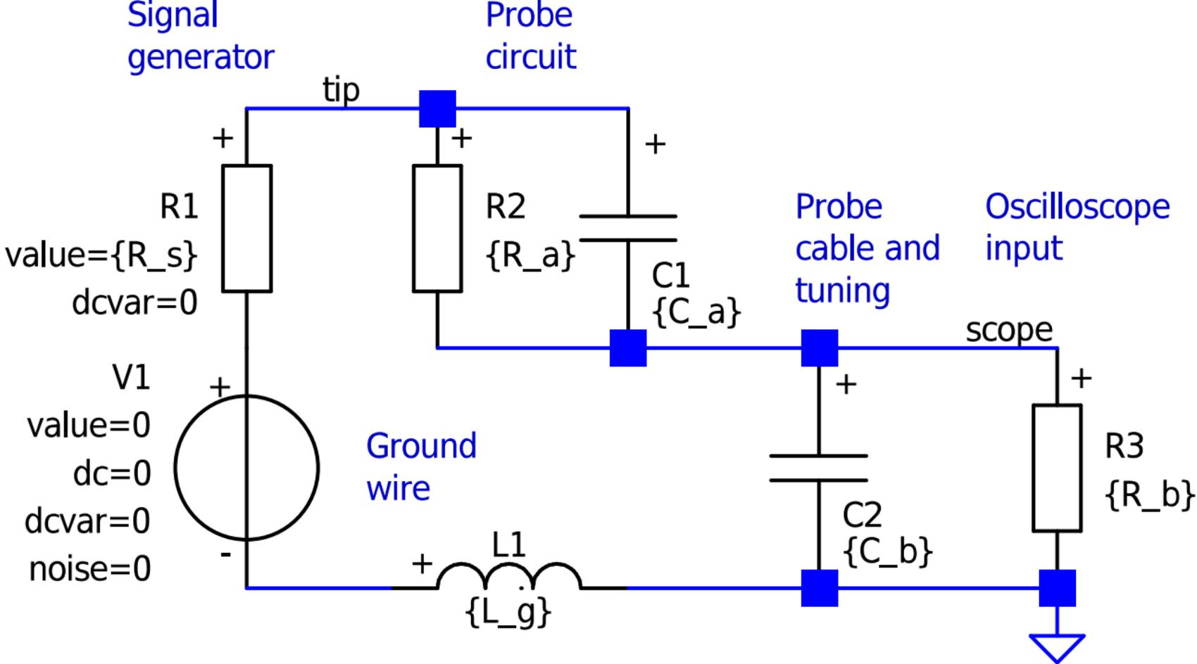
.param A=10 L\_g=10n R\_s=50 R\_a={{(A-1)\*R\_b}} R\_b = 1M C\_a=15p C\_b={{C\_a\*R\_a/R\_b}}
