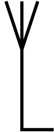
A whip antenna (short rod) is often applied as E-field sensor
