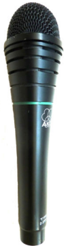
Figure 2.9: A microphone is designed such that its open-circuit output voltage shows the best correspondence with the sound pressure.
