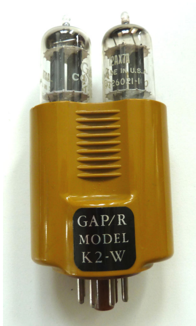
Figure 8.1: K2-W commercial vacuum tube operational amplifier (1952).
