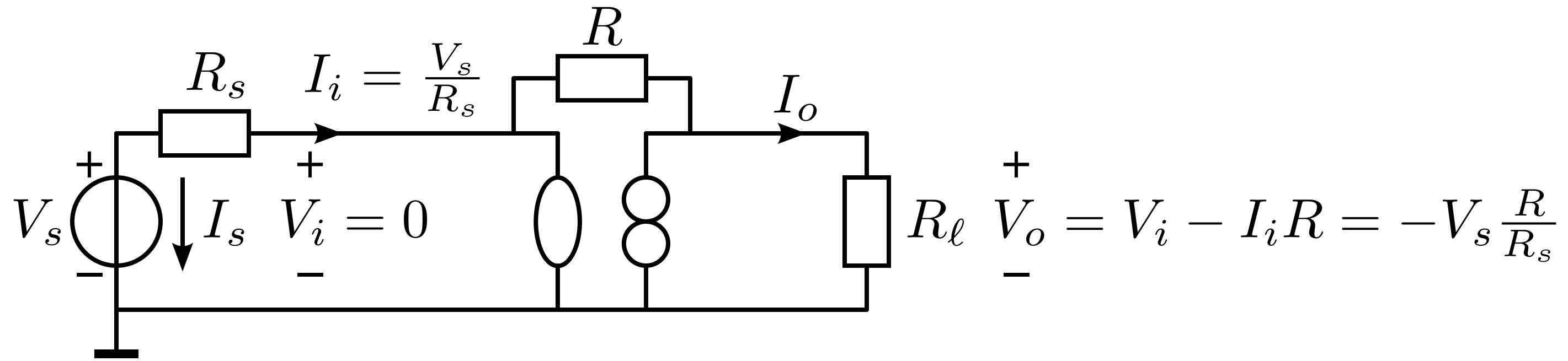
$$A = \lim_{R_\ell \rightarrow \infty} \left( \frac{V_i}{V_o} \right) = 0 \quad C = \lim_{R_\ell \rightarrow \infty} \left( \frac{I_i}{V_o} \right) = \frac{\frac{V_s}{R_s}}{-V_s \frac{R}{R_s}} = -\frac{1}{R}$$
